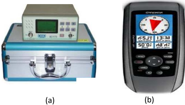
Fig. 3. Picture of (a) the field strength meter (b) GPS meter used
