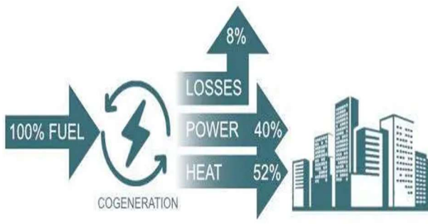
Figure 5. Cogeneration system outputs
