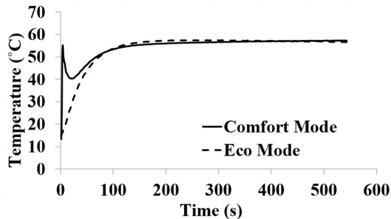
**Figure 3.** DHW outlet temperature comparison between the eco and comfort modes [1].
