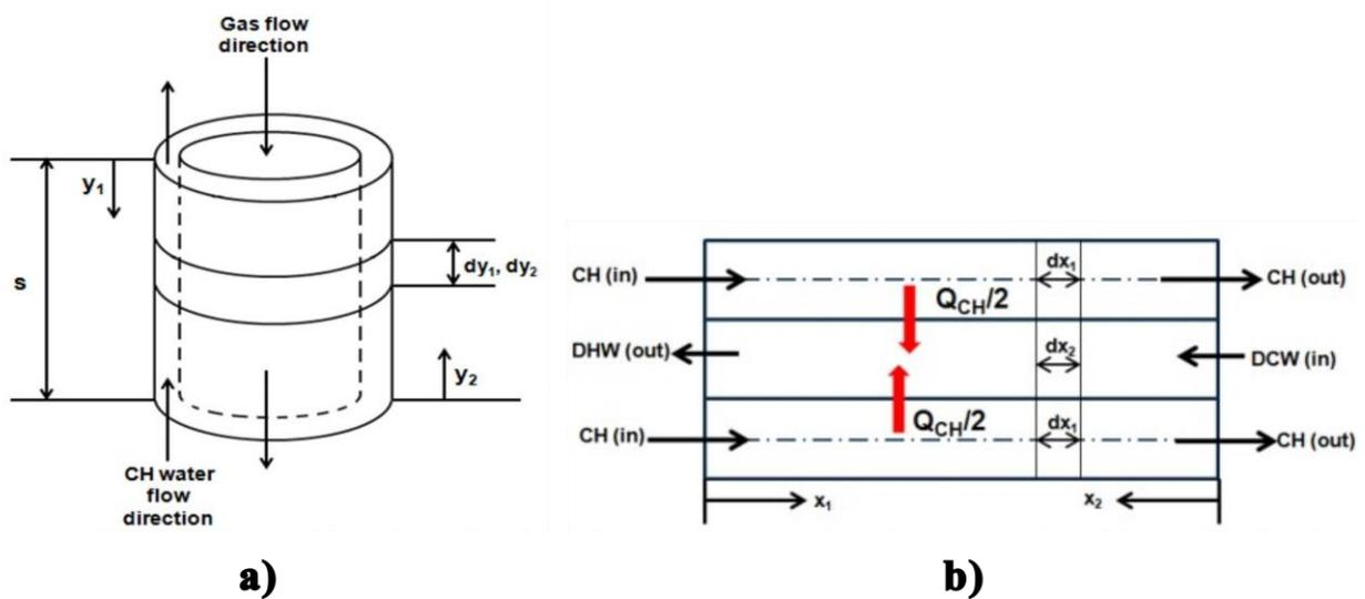
**Figure 4.** Display of the control volumes and water flow directions for (a) the HC and (b) the PHE [1].
