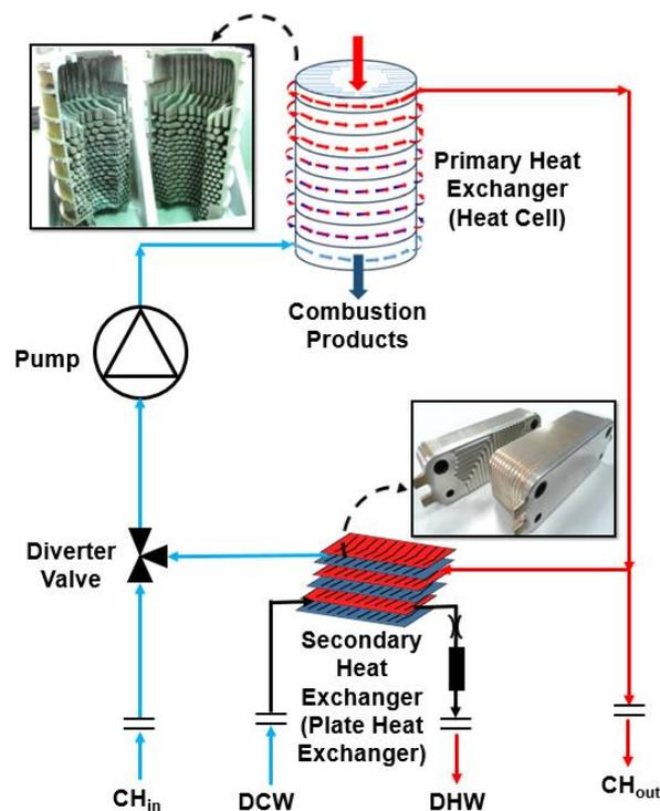
**Figure 1.** Schematic display of the combi boiler heating appliance with the actual views of the primary and secondary heat exchangers.
