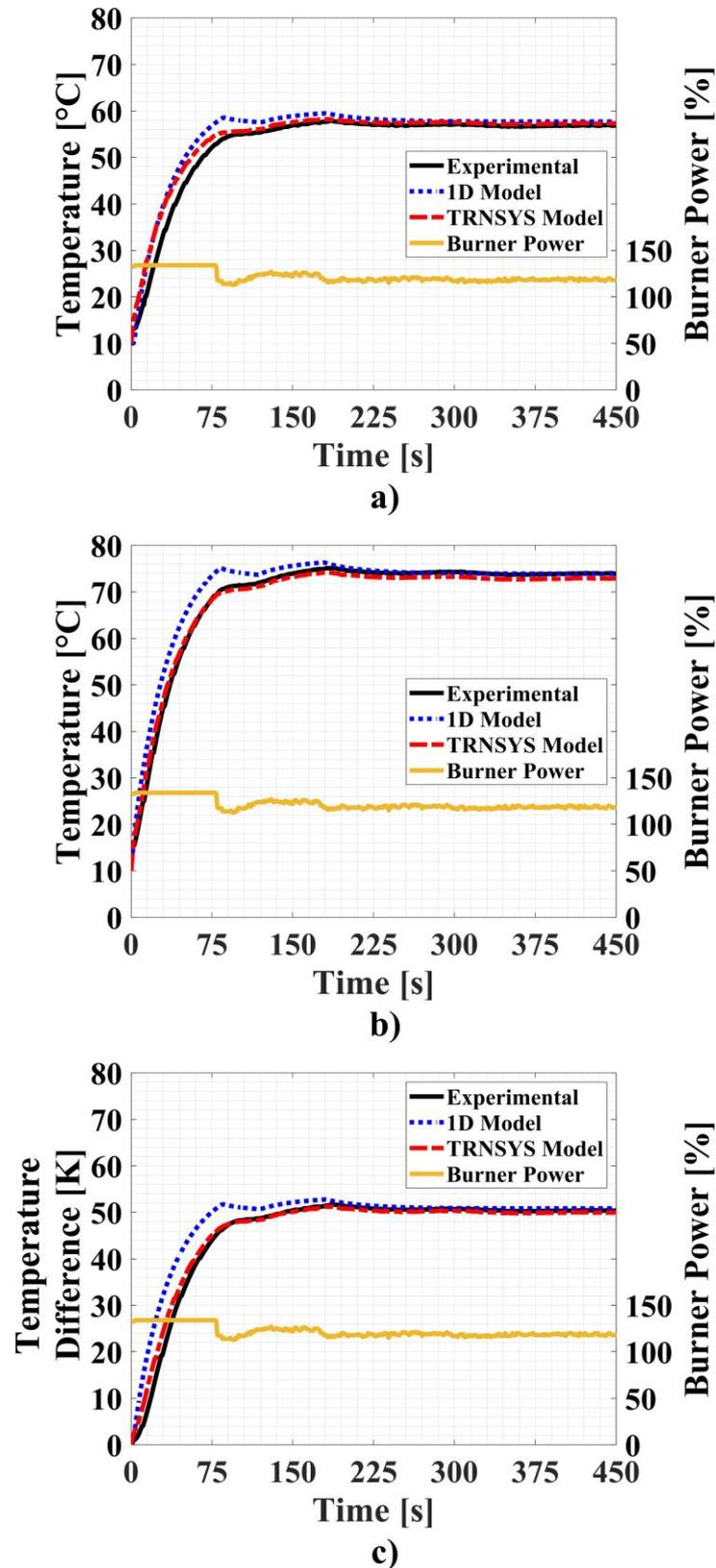
**Figure 9.** Comparison of (a) the CH inlet temperature, (b) the CH outlet temperature, and (c) the DHW inlet and outlet temperature difference among the 1D model, TRNSYS model, and the experimental data for 7 l/min DHW flow rate.
