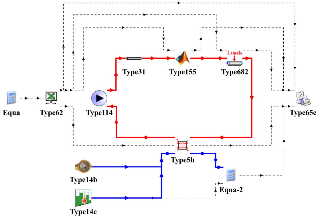
Figure 5. DHW heating circuit model of the combi boiler created in TRNSYS user interface.
