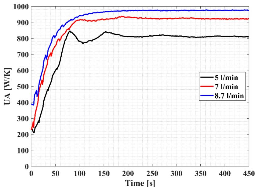
**Figure 6.** Variation of the UA coefficient for the Type 5b-counterflow plate heat exchanger.
