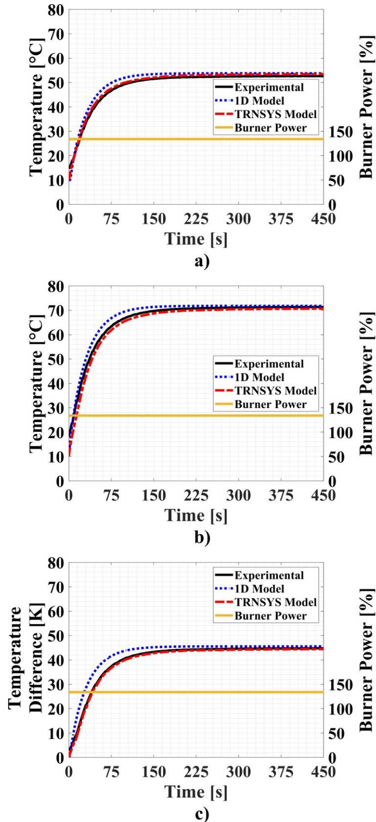
**Figure 10.** Comparison of (a) the CH inlet temperature, (b) the CH outlet temperature, and (c) the DHW inlet and outlet temperature difference among the 1D model, TRNSYS model, and the experimental data for 8.7 l/min DHW flow rate.
