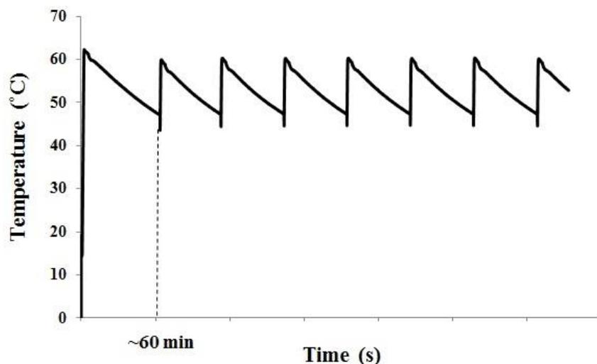
**Figure 2.** Preheat cycles of the CH water in the HC in the comfort mode [1].
