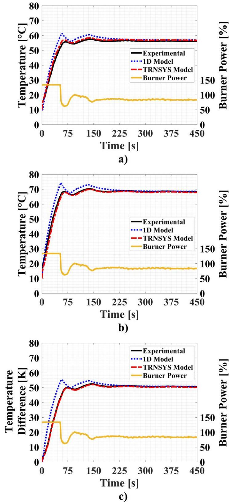
**Figure 8.** Comparison of (a) the CH inlet temperature, (b) the CH outlet temperature, and (c) the DHW inlet and outlet temperature difference among the 1D model, TRNSYS model, and the experimental data for 5 l/min DHW flow rate.
