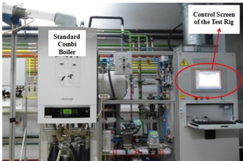
**Figure 7.** Combi boiler test rig [1].
