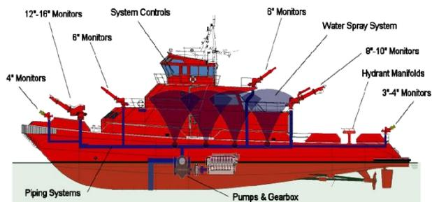
Fig. 10. Fire suppression system ship fire extinguishers (URL 5).
