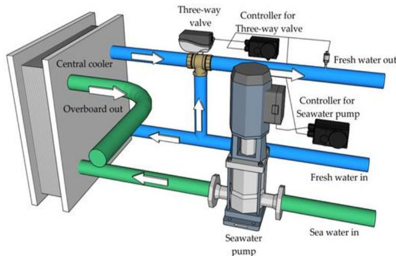
Fig. 4 Configuration of the ship's central cooling system (Lee et al., 2021).
