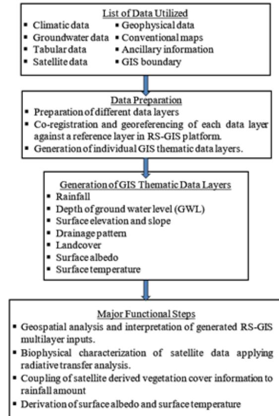
Figure 4. Functional block of planned methodology
