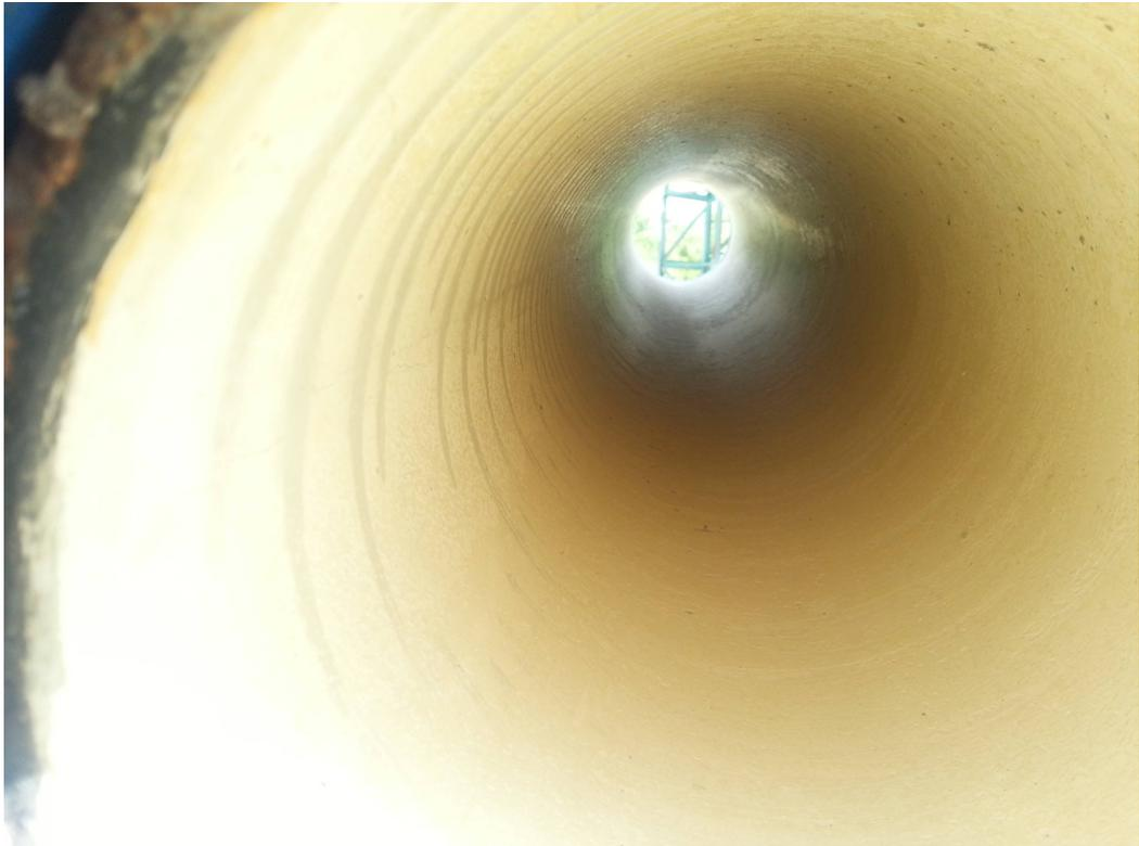
Figure 7: Inner concrete lining after three months test (Ø200) V=13.81 m/s,[22]
