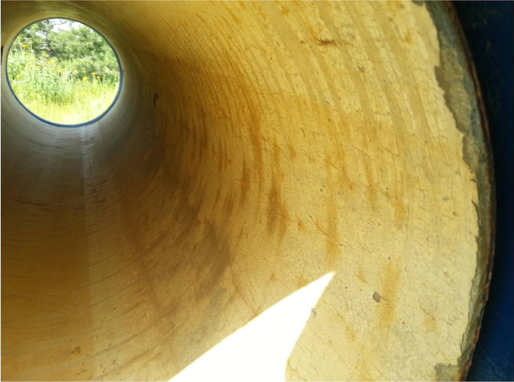
Figure 6: Inner concrete lining after three months test (Ø400) V=3.45 m/s, [22]
