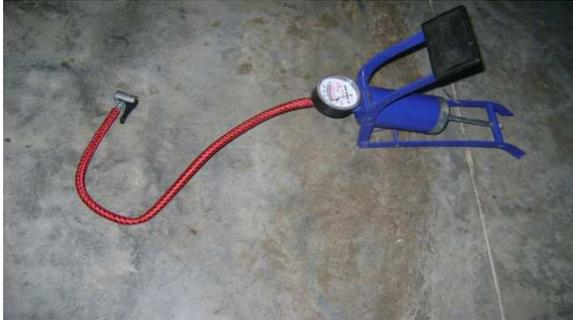
Figure: Foot pumper with pressure gage & air passing pipe.
