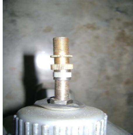
Figure: Air inlet valve.
