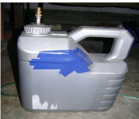
Figure: Cutting fluid tank.
