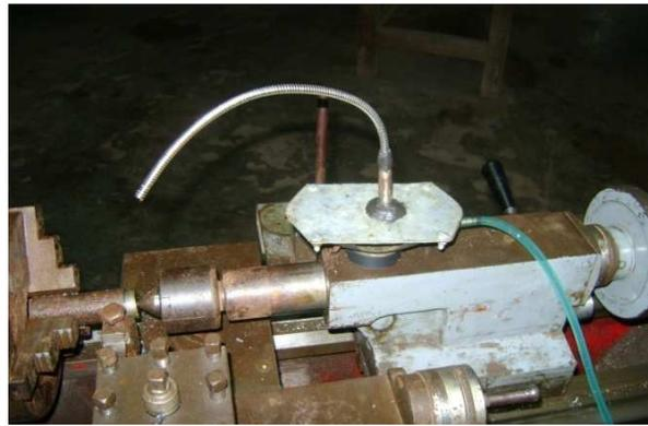
Figure: Magnetic disk post with flexible coil pipe.
