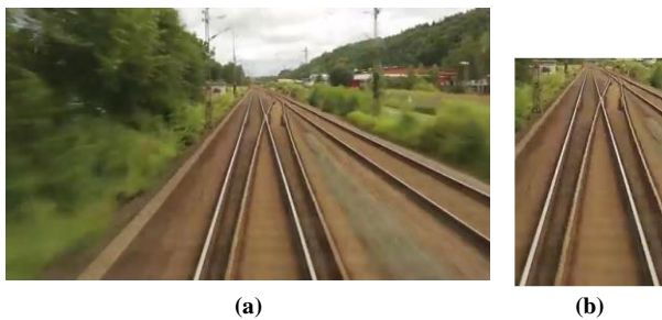
Figure 11. (a) Example railway input image (b) output image for ROI segmentation method
