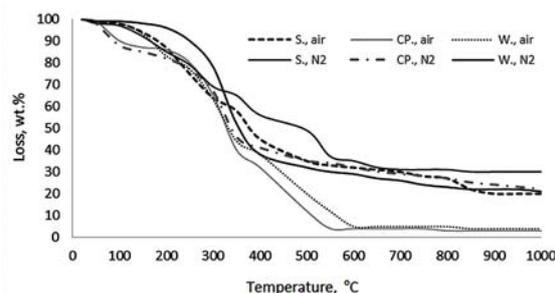
**Figure 2.** Thermogravimetric comparison of feedstock.
