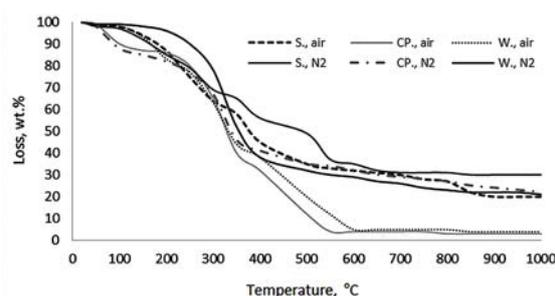
**Figure 2.** Thermogravimetric comparison of feedstock.
