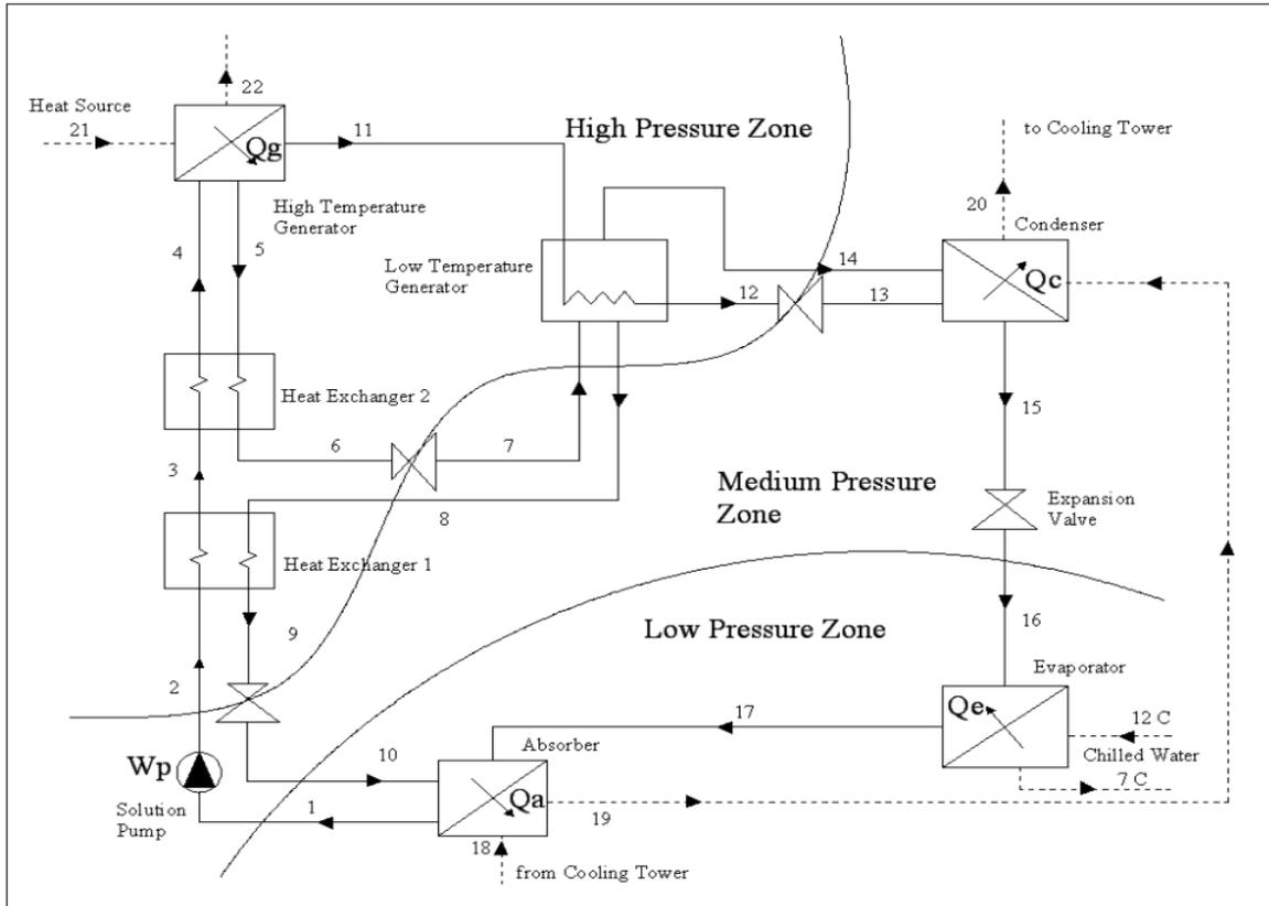
Figure 1. The connection layout of a series flow type double effect absorption chiller [17].
