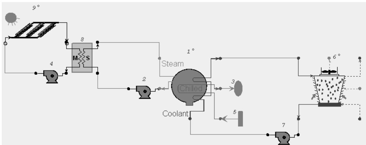
Figure 2. Solar driven absorption cooling system.
