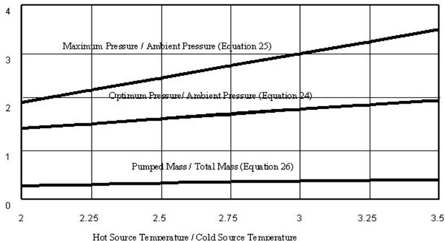
**Figure 3.** Variation of pressure mass ratio with temperature ratio
