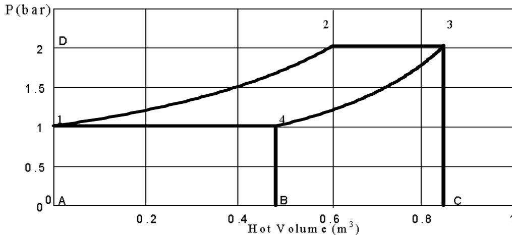
**Figure 1.** Variation of Pressure With Hot Space Volume.
