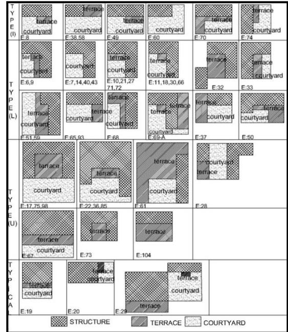
Figure 7. Plan types of two storey structures
