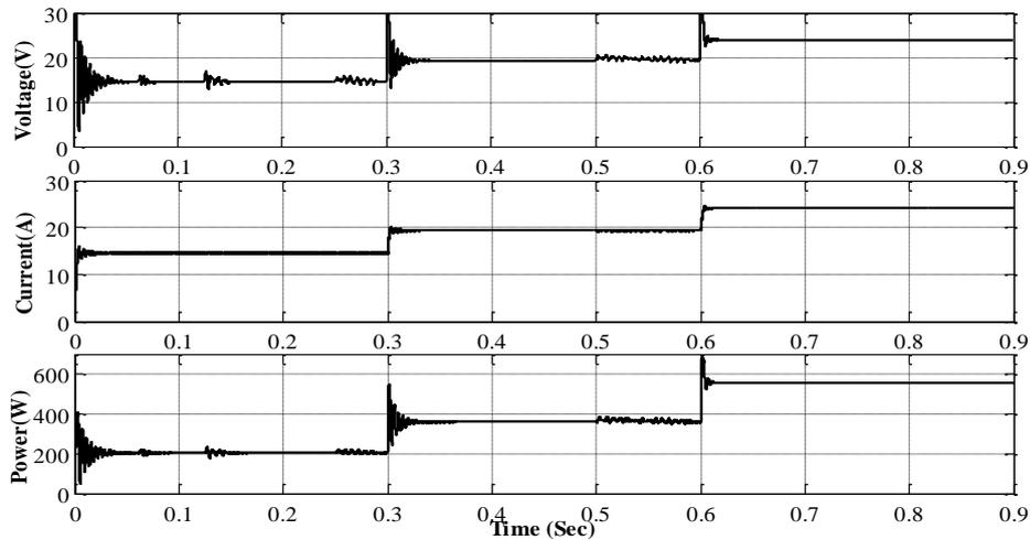
Figure 11. PV panel output voltage, current, and power at different irradiation levels
