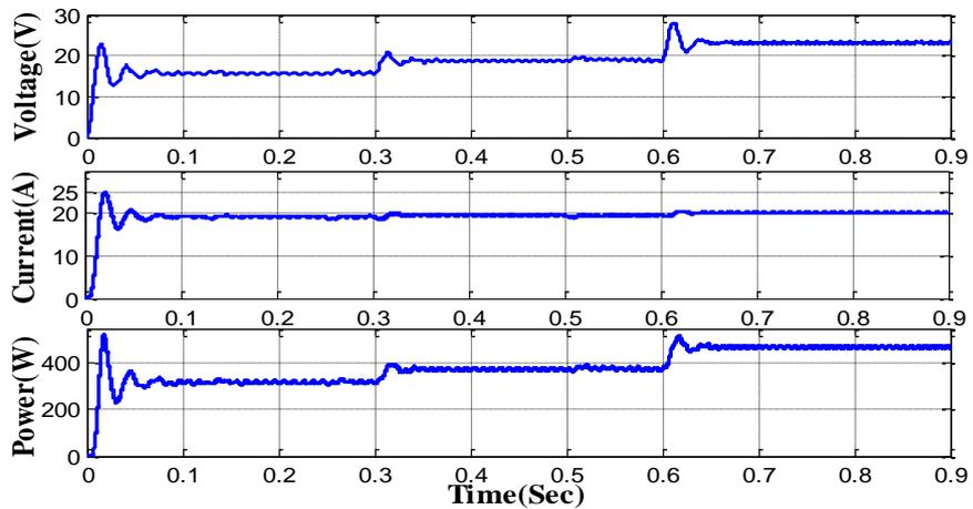
Figure 19. Wind system output voltage, current, and power at different wind velocity levels
