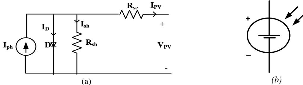
**Figure 3.** (a) PV cell single diode model equivalent circuit, (b) PV cell Symbolic representation
