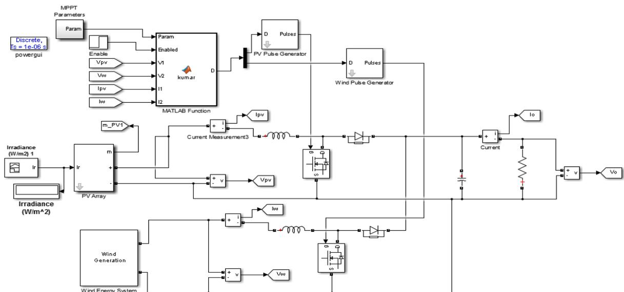
Figure 17. Simulation of hybrid PV and wind system with modified single P&O MPPT technique
