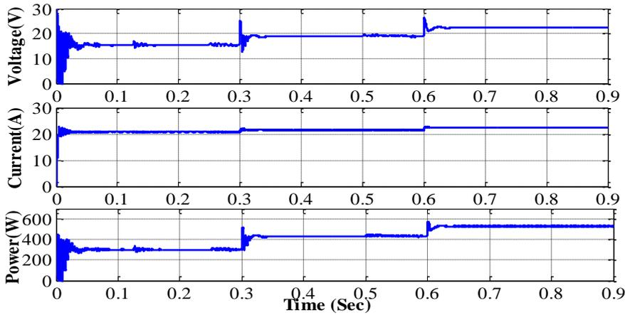
Figure 18. PV panel output voltage, current, and power at different irradiation levels
