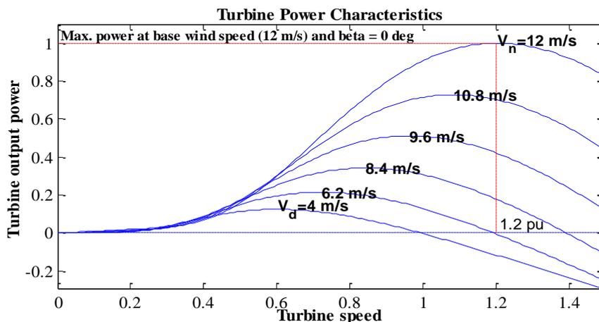
**Figure 5.** Aeolos-H 500W Wind turbine power characteristics
