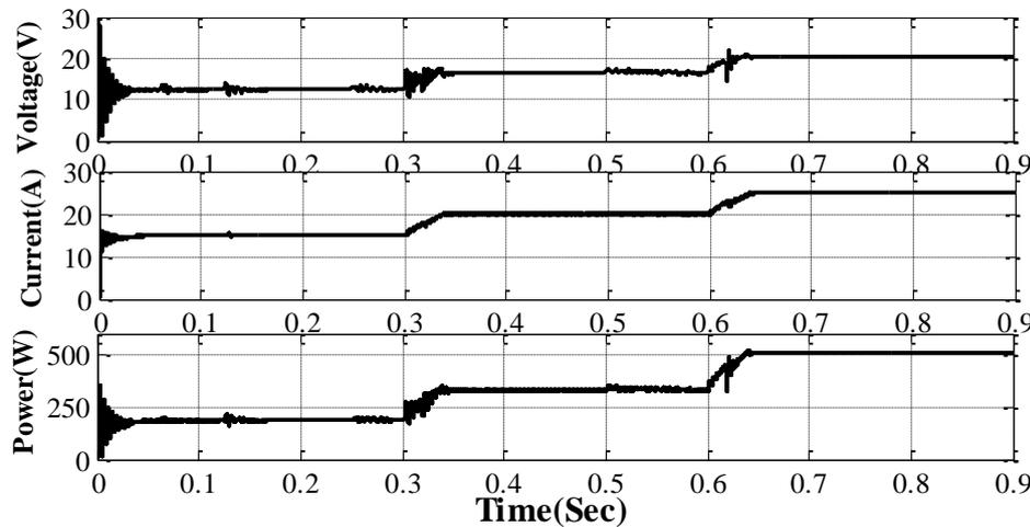
Figure 15. Wind system output voltage, current, and power at different wind velocity levels
