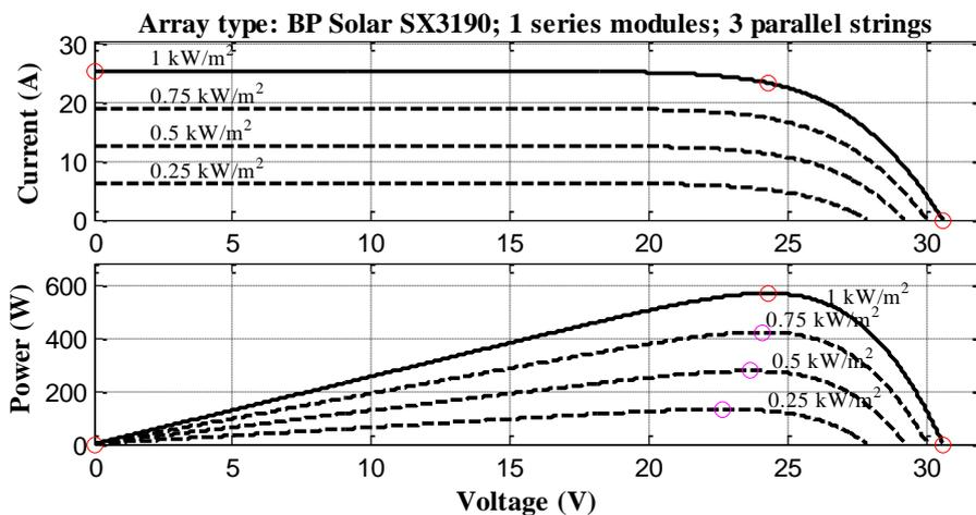
**Figure 4. BP Solar SX3190 model P-V and I-V Characteristics**
