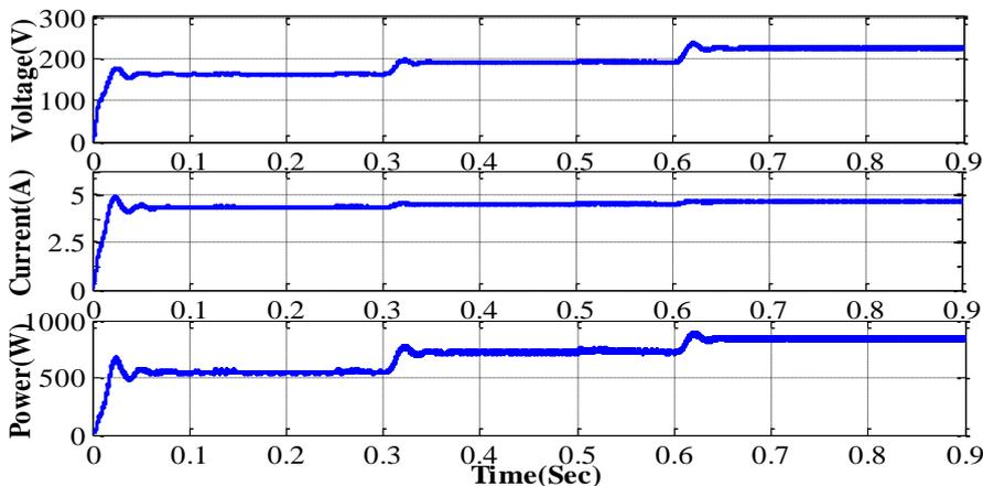
Figure 20. Output DC link capacitor voltage, current, and power
