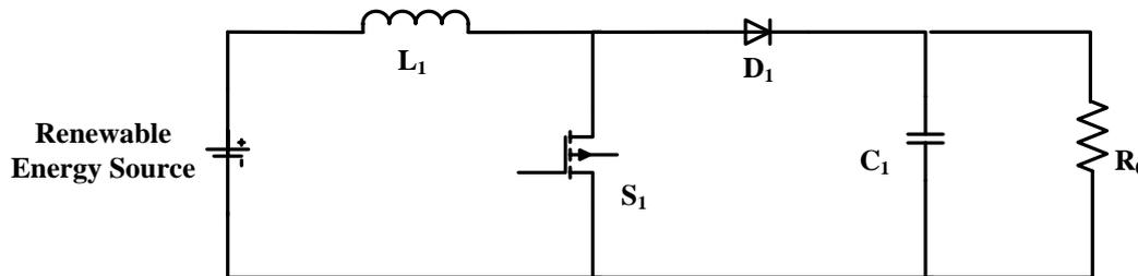
**Figure 6.** Conventional Boost converter circuit
