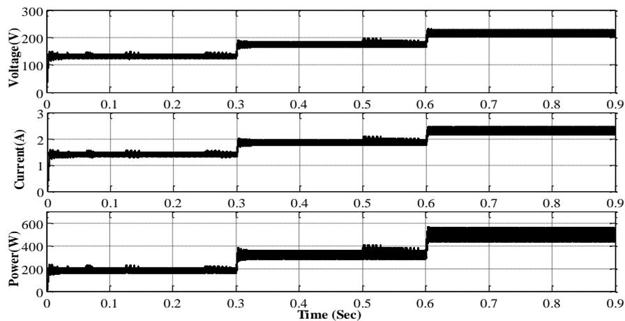
Figure 12. Boost converter output voltage, current, and power
