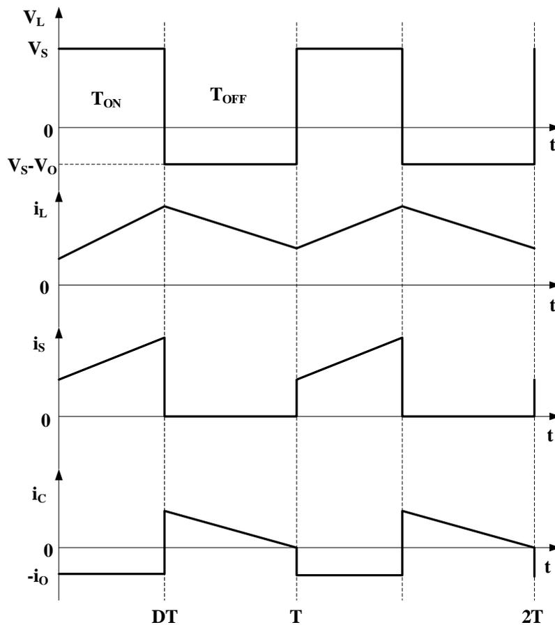
Figure 7. Switching waveform of Boost Converter
