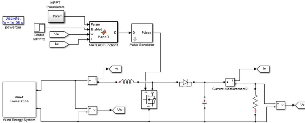
Figure 13. Simulation of Wind system with Boost converter and P&O MPPT
