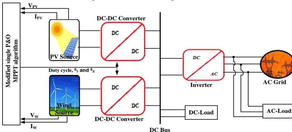
Figure 2. Proposed topology for hybrid PV and wind system with single MPPT
