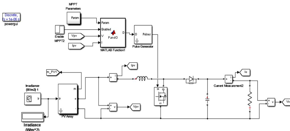
Figure 9. Simulation of PV system with Boost converter and P&O MPPT
