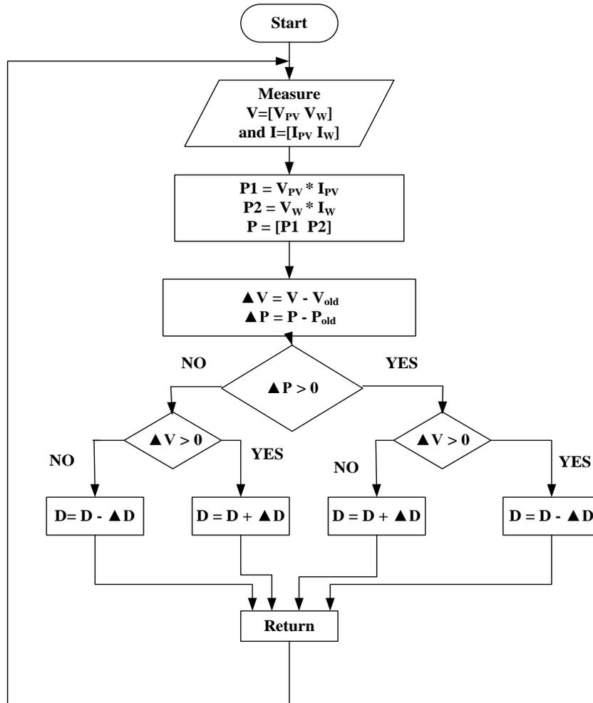
**Figure 8.** Flow chart of modified P&O MPPT for hybrid system
