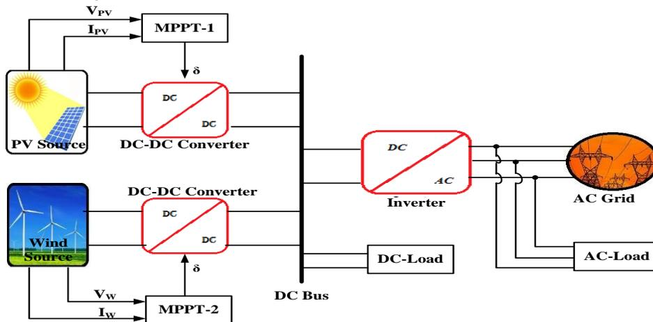
Figure 1. Basic topology for hybrid PV and wind system
