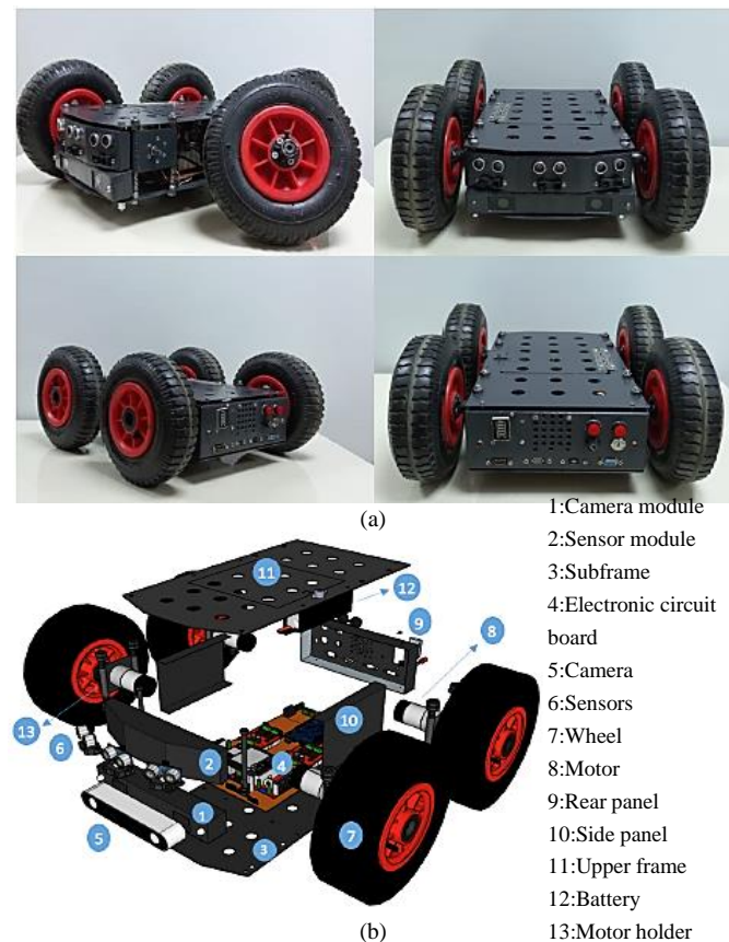
Figure 1. (a) Views of the SMaRt from different angles and (b) the off-the-shelf 3D model rendered in SketchUp.
