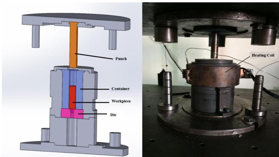
Figure 2. CAD model and view of die set-up
