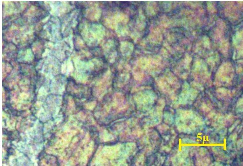
*Figure 3. Optical microscope view of microstructure after deformation*
