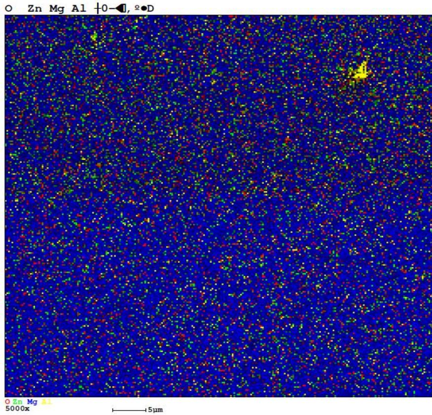
Figure 4. EDAX mapping photo of microstructure before deformation (green:Zn, blue:Mg, yellow:Al)
