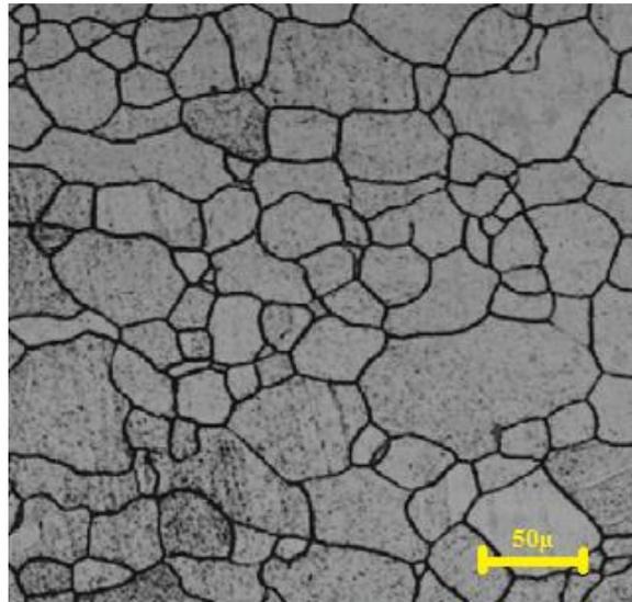
Figure 1. Optical view of microstructure before deformation
