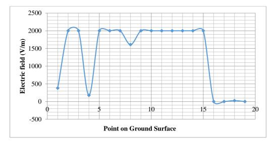
Figure 5: Waveform of the electric field strength from the left side of transmission tower.
