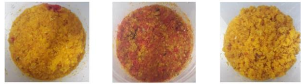
Fig.2. Samples of urease test images (From left to right: well-cooked, undercooked and overcooked).
