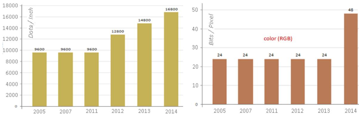
Figure 3. a) Evolution of scanner read resolutions.
