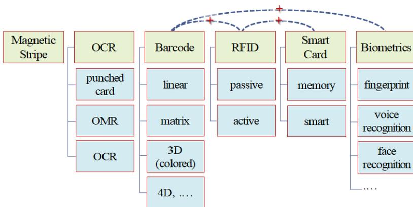
**Figure 1.** Barcodes in auto-ID technologies.
