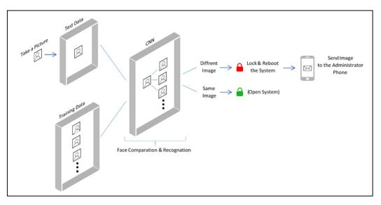
Figure 4. Block diagram of the developed system.
