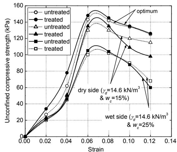
Figure 6. Effect of cutting stone slurry waste on the unconfined compressive strength for soil-3 at the optimum, dry and wet side of the optimum
