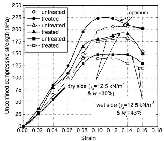
Figure 4. Effect of cutting stone slurry waste on the unconfined compressive strength for soil-1 at the optimum, dry, and wet sides of the optimum
