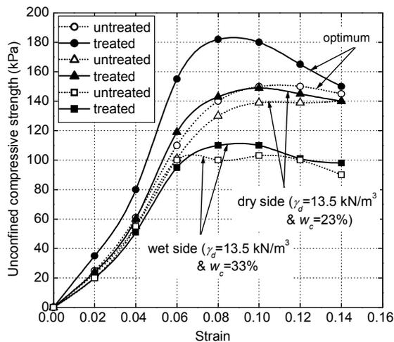
Figure 5. Effect of cutting stone slurry waste on the unconfined compressive strength for soil-2 at the optimum, dry, and wet sides of the optimum
