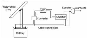
Figure 1. Schematic presentation and components of the bird scarer.
