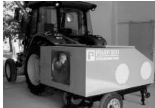
Figure 1. Tractor PTO test system.
