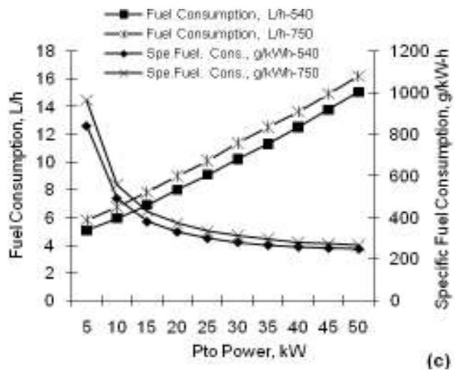
Figure 3 – Fuel consumption and specific fuel consumption depending on the loads applied to the tractor PTO at 540 and 750 rpm operations (a) JD 5625, (b) MF 3085, (c) NH TD85.
