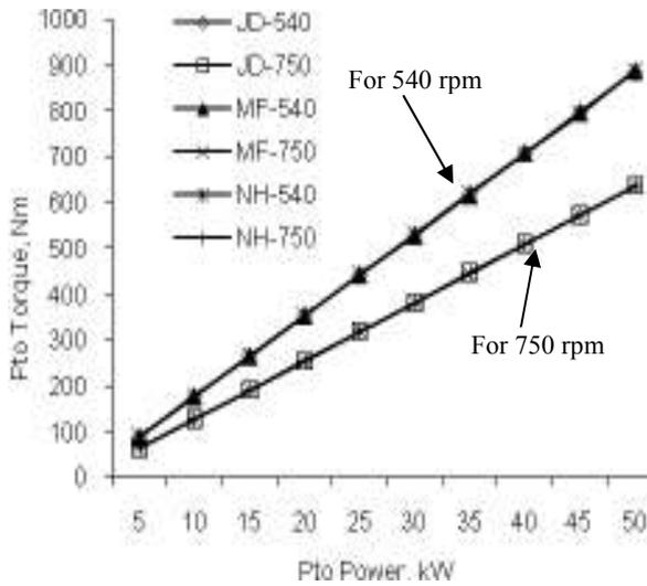
Figure 2 - PTO torque depending on the loads applied to the tractor PTO at 540 and 750 rpm operations.
