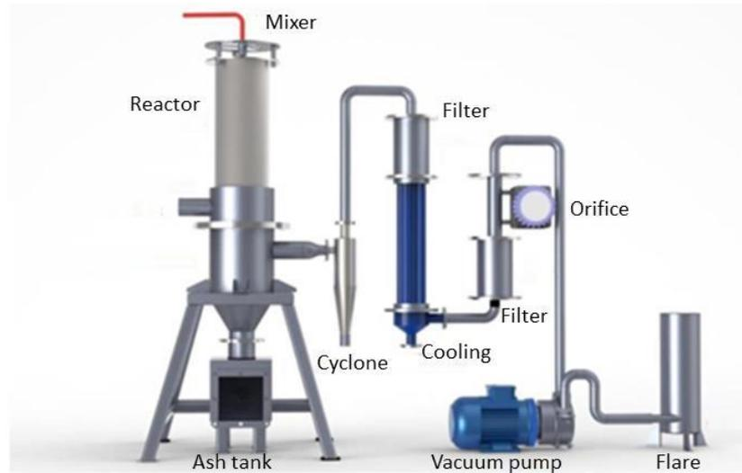
**Figure 1- The gasification system units**
