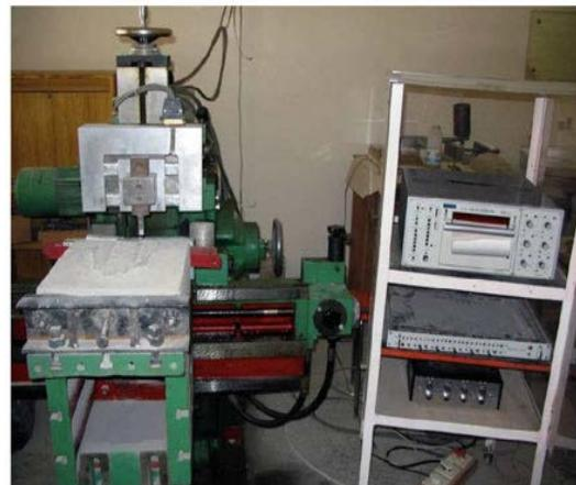
Figure 3. Setup for the rock cutting experiment and the rock sample test
