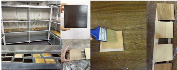
Figure 1. Varnishing of test samples
