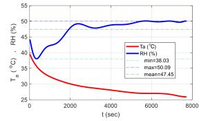
Figure 2. Bus Internal Temperature and RH inside the Bus
