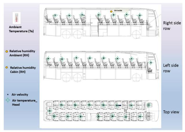
Figure 1. Measurement Points on the Pasenger Bus
