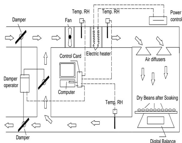
Figure 1. Drying system (Kurutma sistemi)
