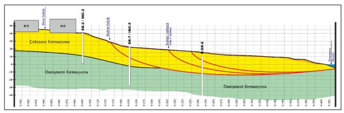
Figure 2. Simplified geologic section of landslide area along the section-4.
