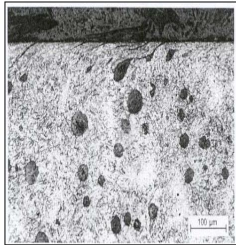
Figure 3. Surface microstructure of the ADI test sample after roll / slip testing at  $F_N = 3935$  N (Madler, 2000)
