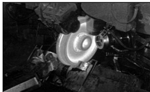
Figure 2. Wheel rolling equipment (Vantuono, 2000)
