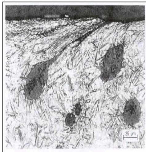
Figure 4. Surface microstructure of the ADI test sample after roll / slip testing at  $F_N = 5665$  N (Madler, 2000)
