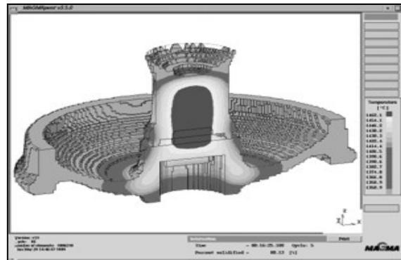
Figure 1. Solidification pattern in graphite mould (Vantuono, 2000)
