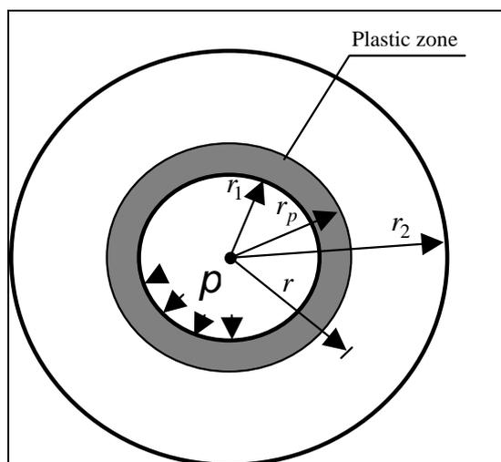
Figure 1. An aluminum disc with a hole under internal pressure,  $p$ , has a unit thickness, inner radius,  $r_1 = a = 50$  mm, outer radius,  $r_2 = b = 100$  mm, radius at yield,  $r_p$  and radius at any point,  $r$ , and all its edges are free
