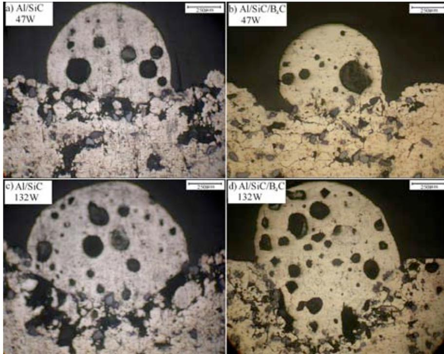
**Figure 2. Optical micrographs of Al/SiC and Al/SiC/B<sub>4</sub>C MMCs laser welded at different power levels.**
