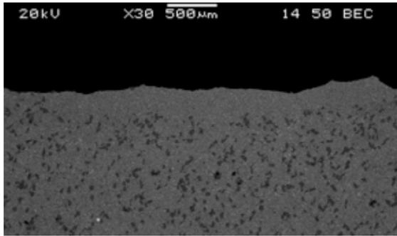
Figure 4. SEM image of GTA weld bead on the Al/SiC material.
