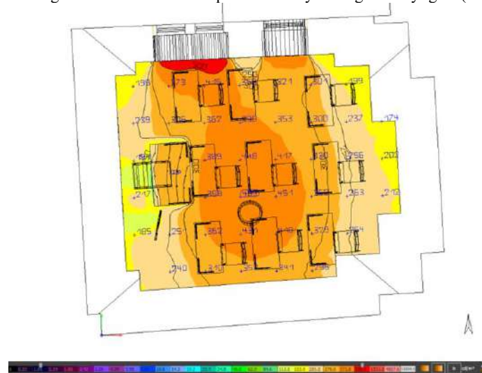
Figure 9: Contour diagram for classroom “2” optimization by adding pipe light (93.8lux to 304 lux)
