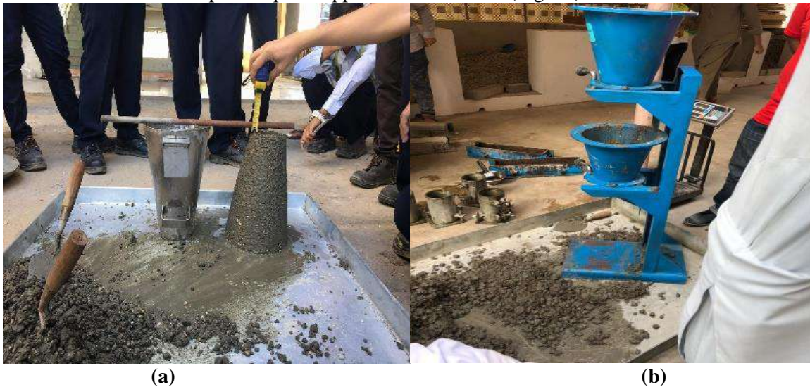
Figure 1: a) show Slump test apparatus and b) show Compacting test apparatus
