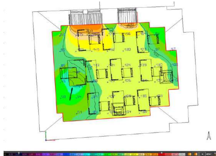
Figure 8: Contour diagram for classroom “2” optimization by adding two skylights (93.8lux to 122 lux)
